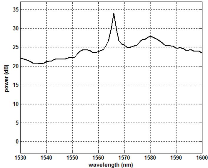
Figure 5: output spectrum of the supercontinuum obtained with the OTDR
