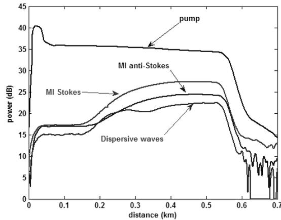
Figure 3: OTDR traces for the most noticeable feature in the spectrum
