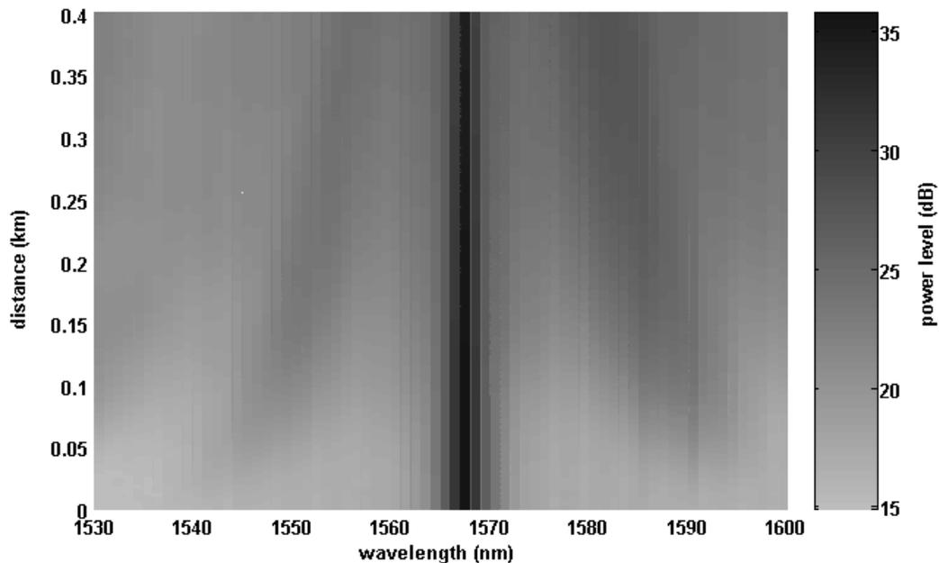
Figure 4: map of the supercontinuum generated in the fiber
