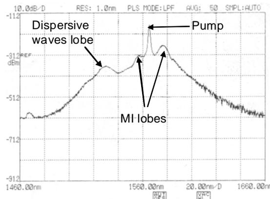
Figure 2: output spectrum of the SCG obtained with an optical spectrum analyzer
