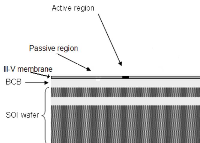
Figure.1 The layer stack of the membrane platform
