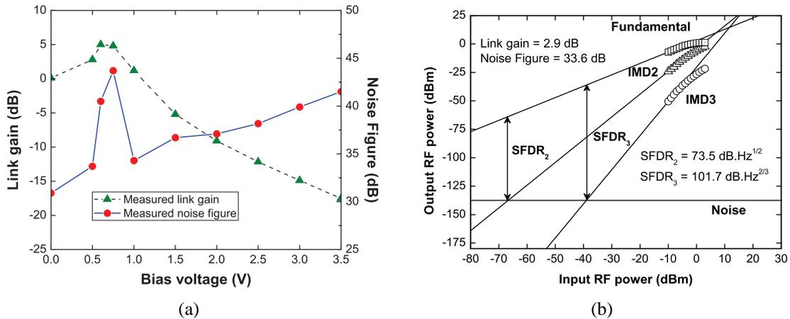
Figure 3: Measured figure of merits of the optically amplified APL. (a) Link gain and NF (b) SFDR at  $V_B = 0.5$  V.
