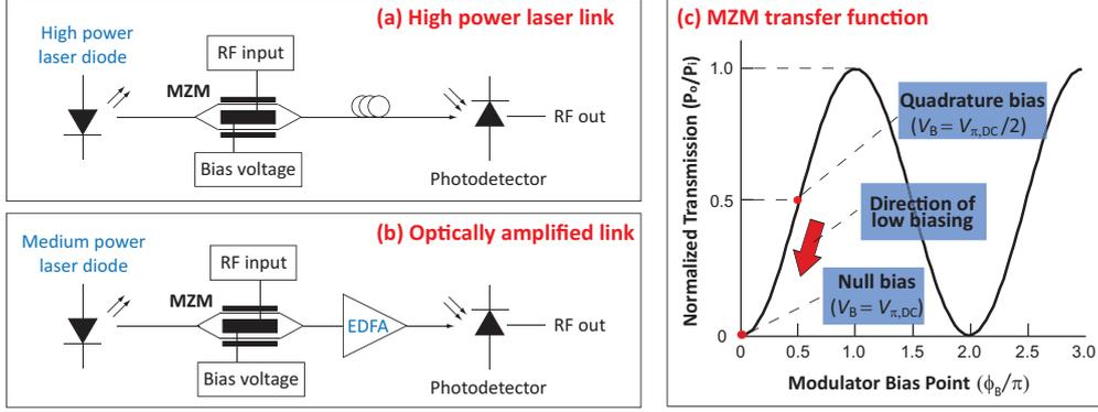
Figure 1: (a) High power laser link, (b) optically amplified link, (c) MZM transfer function.
