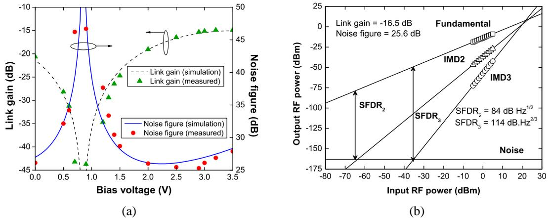
Figure 2: Measured figure of merits of the high power laser APL. (a) Link gain and NF (b) SFDR at  $V_B = 2.0$  V.
