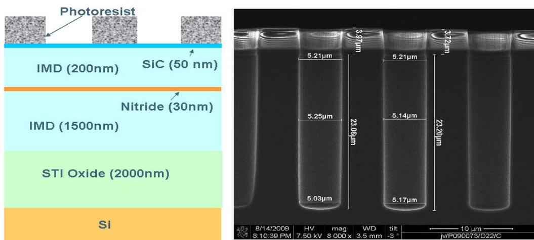
**Figure 2: Stack Structure for Photonics Layer; TSV Etches**
