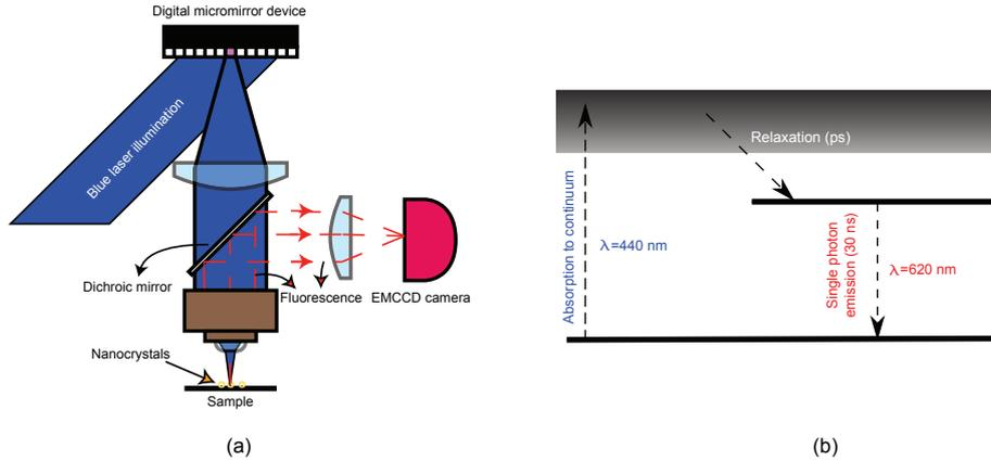
Figure 1: (a) Outline of the experimental setup. (b) Simplified “3-level” approximation of the CdSe/ZnS electro-dynamics.
