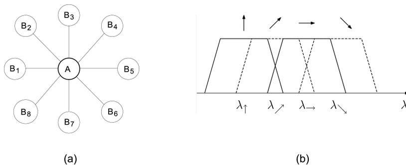
Figure 3: (a) A quantum cryptography network with a central server  $A$  and  $n$  nodes  $B_i$  ( $i \in \{1, \dots, n\}$ ). (b) Wavelength coding for quantum cryptography.
