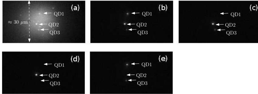
Figure 2: (a) To observe the entire field of view, all the micro-mirrors of the array are switched on. (b) Only mirrors addressing quantum dots QD1, QD2, and QD3 are switched on. (c) QD2 and QD3 are on, QD1 is off. (d) Only QD2 is on. (e) QD1 and QD3 are on, QD2 is off.
