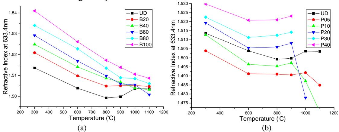
Figure 2. Refractive index changes of (a) B-doped and (b) P-doped SiON layers as a function of annealing temperature
