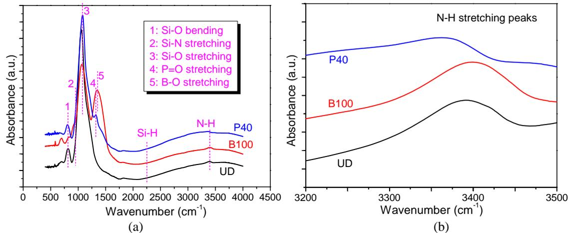
Figure 3. (a) Comparison of full FTIR spectra of three as-deposited samples; with indication of the positions of some absorption peaks under our interests, (b) Magnification of spectral section containing the absorption peaks caused by stretching of N-H bonds
