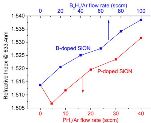
Figure 1. Refractive indices of as-deposited layers as a function of the B<sub>2</sub>H<sub>6</sub>/Ar and PH<sub>3</sub>/Ar flow rates
