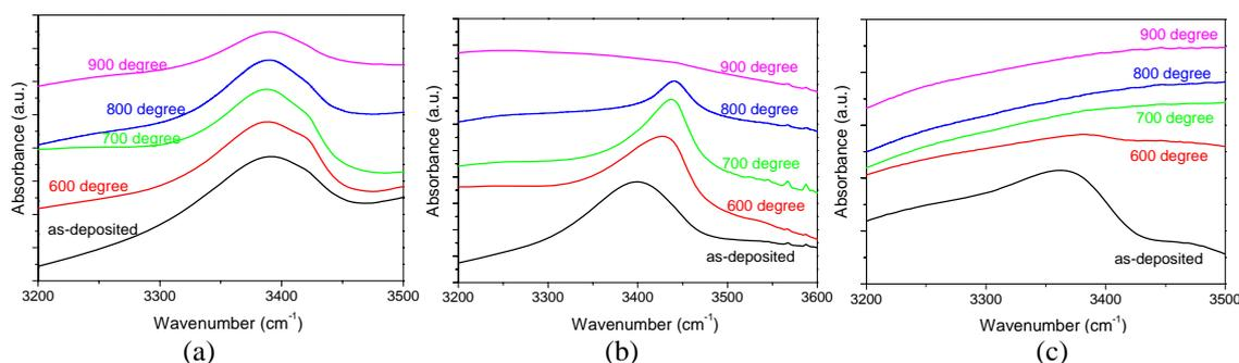
Figure 4 Reduction of N-H absorption peaks upon anneal treatment at varied temperatures: (a) undoped sample UD, (b) B-doped sample B100, and (c) P-doped sample P40
