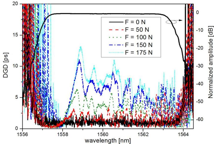
Fig. 3 : Experimental results: DGD evolution of a CFBG for different transversal loads
