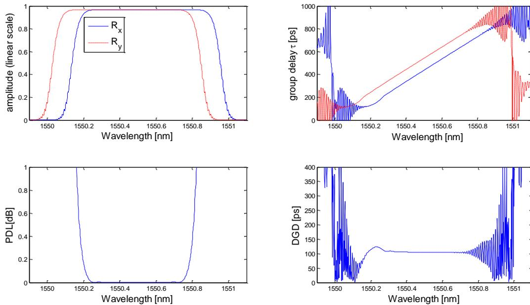
Fig. 1 : (up) Amplitude and phase response (group delay) for the two CFBG eigenmodes; (down) the corresponding PDL and DGD wavelength dependencies
