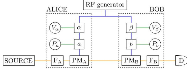
Figure 2: Second experimental setup. The optical part of the experiment consists of a classical broadband source sent through frequency filter  $F_A$ , a polarization controller (not shown), a modulator with parameters  $(a, \alpha)$ , a modulator with parameters  $(b, \beta)$ , and filter  $F_B$ . A photodetector  $D$  measures the optical power.
