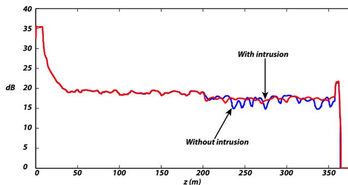
Figure 2. POTDR traces evolutions with intrusion and without intrusion
