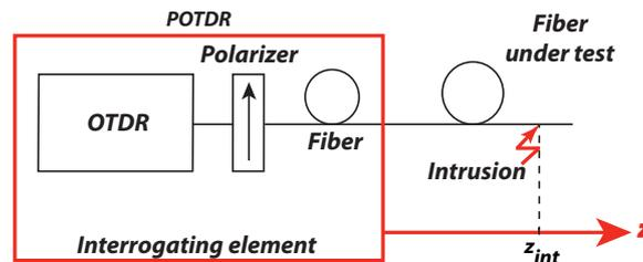
Figure 1. Intrusion set-up
