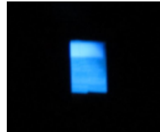
Figure 5 - INP chip glowing due to proton induced fluorescence.
