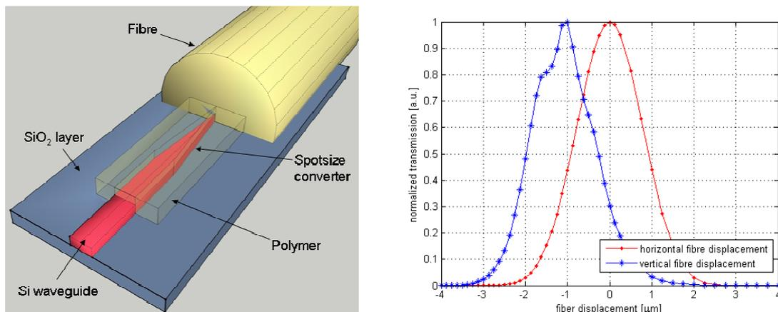
**Figure 1: artist impression of laterally tapered spot size converter design (left) and FDTD simulations of fiber displacement with respect to the spot size converter (right)**
