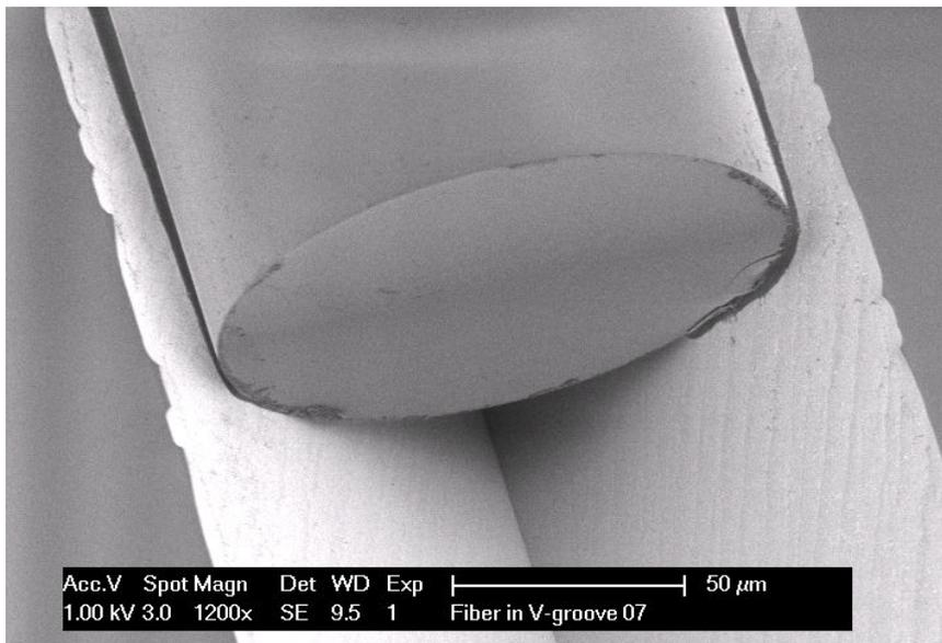
**Figure 3: SEM image of fabricated v-groove with glued fibre**
