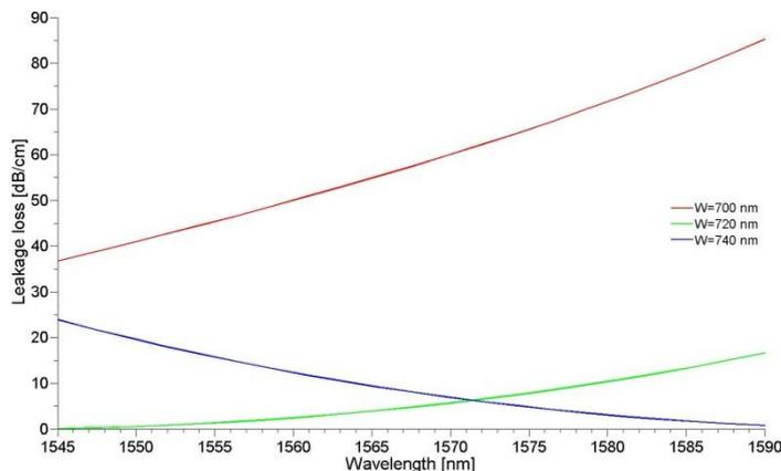
Figure 5: Variation of the Leakage loss with wavelength for fixed ridge waveguide widths.
