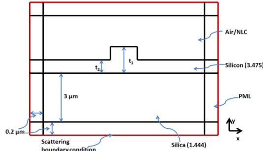
Figure 3: Rough sketch of the simulation set-up.
