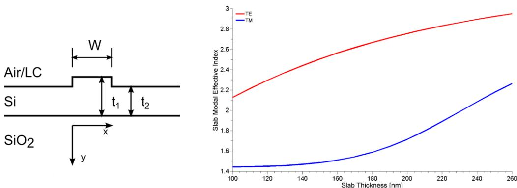
Figure 1: (Left) Problem geometry, the positive z-direction is perpendicular to the page. (Right) Effective index versus slab thickness for an SOI slab waveguide. Plot is obtained using a fully vectorial finite element solver; the operating wavelength is 1550 nm.
