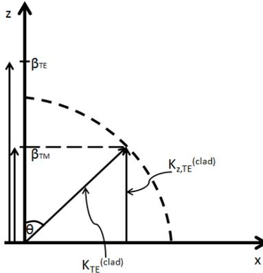
Figure 2: K-vector diagram showing how a TM-like mode can become phase matched to a TE slab mode propagating in the lateral cladding
