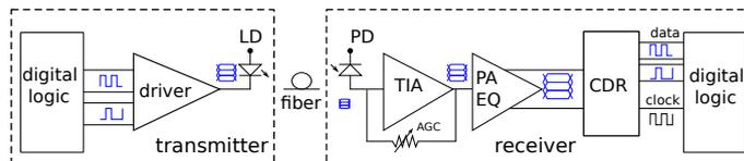
**Figure 2:** Architecture of a 4-PAM optical communication system
