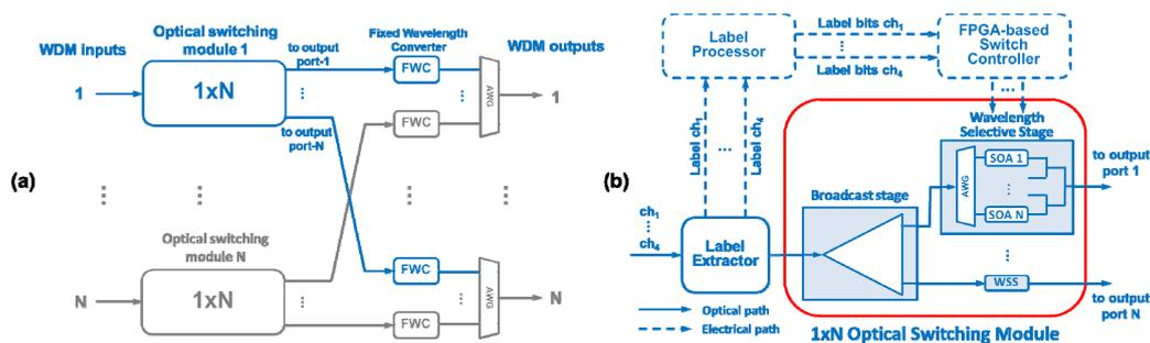
Fig. 1: WDM modular OPS architecture (a) and optical switching module implementation (b)
