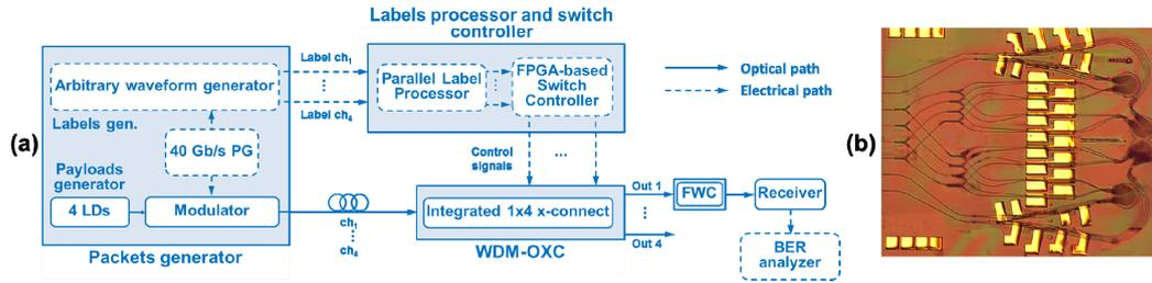
Fig. 2: experimental set-up (a) and photograph of the 4x4 integrated optical cross-connect (b).
