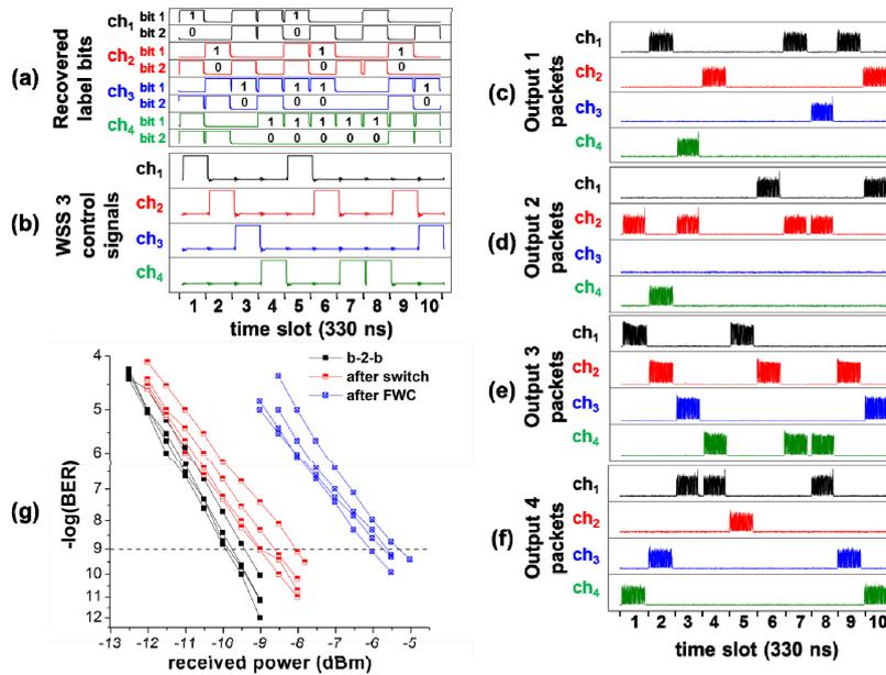
Fig. 3: recovered label bits (a), control signals for WSS 3 (b), output packets time traces (c-f) and BER curves in back-to-back (b-2-b), after switching and after fixed wavelength conversion (g).
