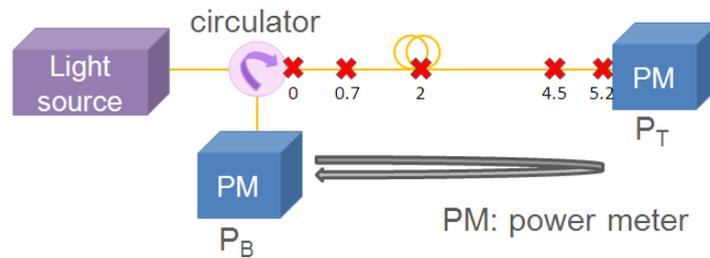
Figure 5: Experimental set up of TRA based on a single fiber
