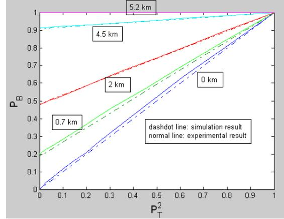
Figure 4: experimental result and simulation result for various loss locations
