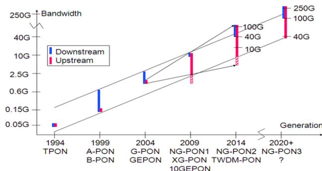
Figure 1: Capacity trend for PON systems [1]
