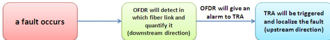
Figure 2: flow chart of the final monitoring method
