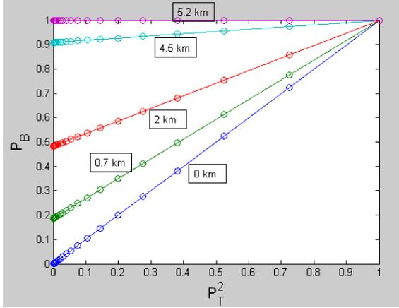
Figure 3: TRA simulation result for various loss locations
