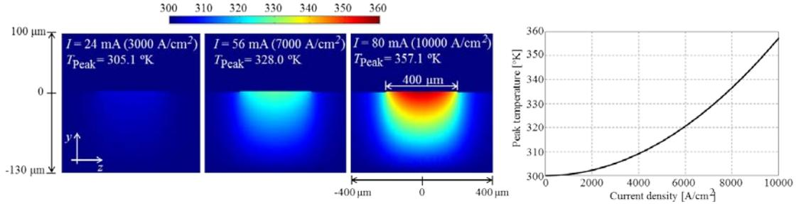
Fig. 2: (left) Temperature distribution in the  $yz$  cross section for three values of injected current, (right) Peak temperature vs injected current density in a single SOA.
