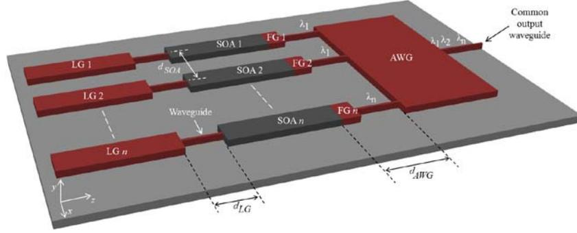
Fig.1: Schematic representation of a multiwavelength transmitter. The distance between the edge of the  $i$ -LG and the  $i$ -SOA is  $d_{LG}$  while the distance between the edge of the  $i$ -LG and the AWG is  $d_{AWG}$ .  $d_{SOA}$  is the distance between the vertical center of two consecutive SOAs. All the SOAs considered in the multichannel transmitter have the same geometrical dimensions.
