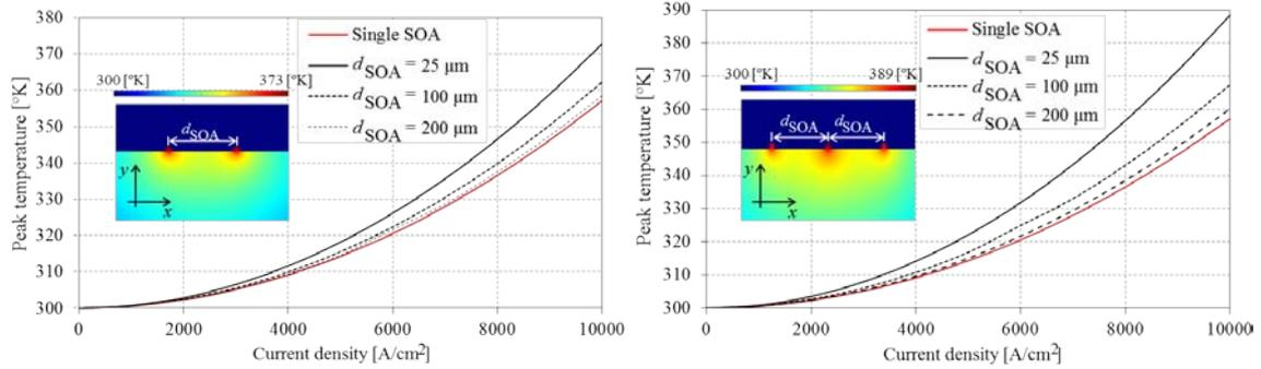
Fig. 3: Behavior of the peak temperature as function of the distance between (left) two SOAs and (right) three SOAs.
