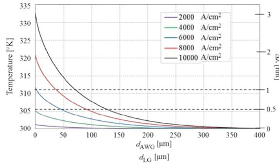
Fig. 3: Temperature distribution in  $z$  direction from the  $z$ -edges of the SOA.
