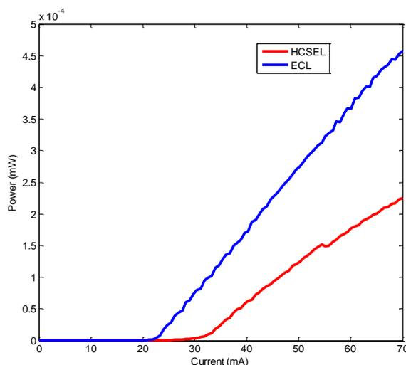
Fig. 4 – I-P characteristics of HCSEL and ECL devices.
