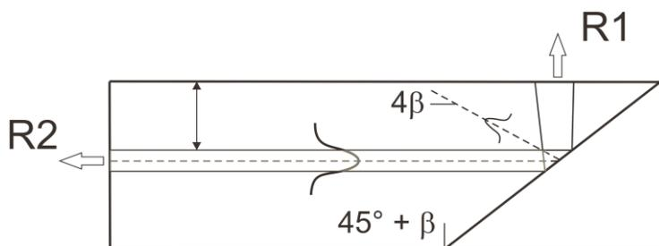
Fig. 3 – Schematic of the vertical coupler output.
