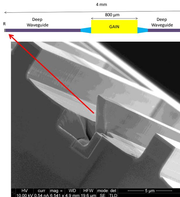
**Fig. 1 – Schematic of the extended cavity laser (top) and SEM picture of the 45° mirror fabricated.**
