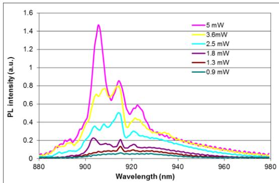
Fig. 6. PL spectra of InP pillars grown on pattern a of Fig. 2 under pulsed pumping. Sharp peaks start to build up when pumping power is increased.
