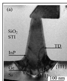
Fig. 1 TEM photo of a typical InP pillar on silicon. Threading dislocations (TD) are terminated by the high aspect ratio SiO<sub>2</sub> trench.
