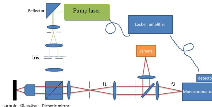
Fig. 3 A schematic diagram of the micro-PL setup
