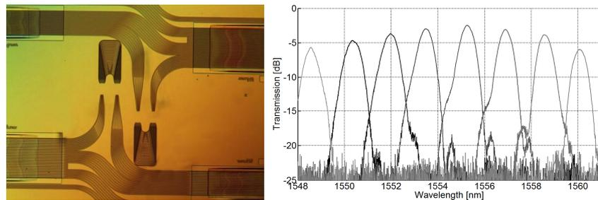
**Figure 4:** Image of fabricated chip containing 84 SSCs and measured AWG transmission
