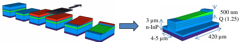
**Figure 1:** Fabrication of a vertical taper using a raster mask in proximity
