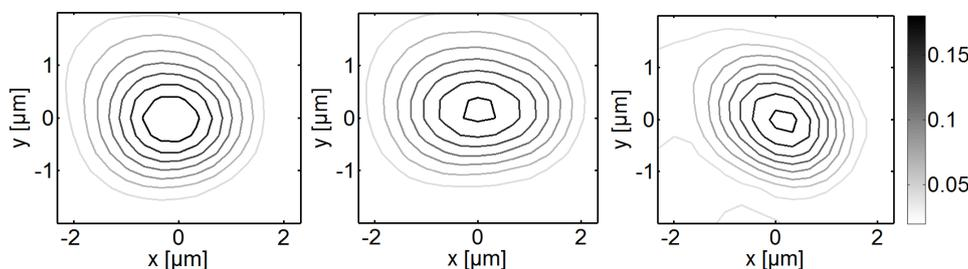
**Figure 2:** Modes of a  $4 \mu\text{m}$  wide FMW,  $5 \mu\text{m}$  wide FMW and  $2.5 \mu\text{m}$  MFD lensed fiber respectively
