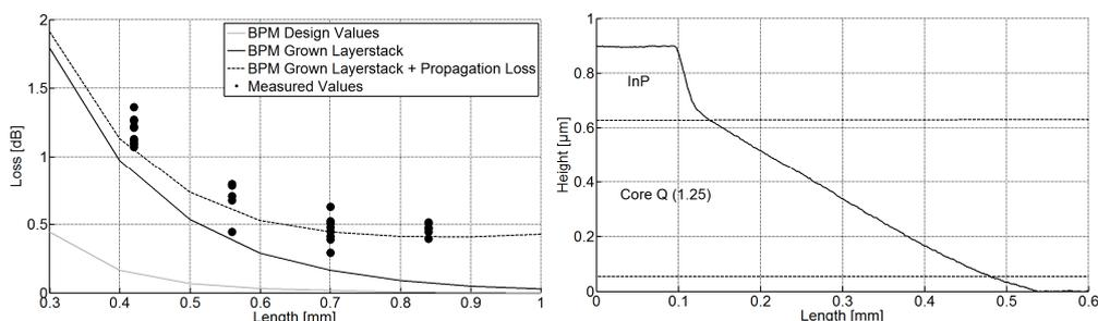
**Figure 3:** Extracted loss of the vertical taper and fabricated ramp indicating the core layer
