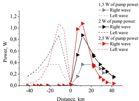
Fig. 1. Longitudinal power distribution for the first Stokes wave in the center-pumped symmetrical configuration at different pump power levels (1, 2 and 2.5 W).
