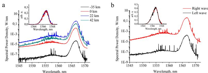
Fig. 2. (a) Spectra of right wave at specific pump power of 2 W at different points of the fiber span. (b) Right and left waves spectra at 22 km point, having the same shape. The normalized spectra in linear scale are shown in insets.
