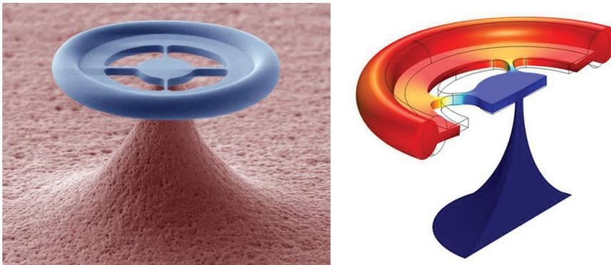
Figure: SEM image of a toroid resonator and the optomechanical coupling between the optical and mechanical degree of freedom mediated by radiation pressure.
