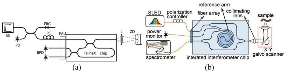
**Figure 2:** Schematic layout of the OCT setup incorporating the TriPleX™ chip (a) AMC measurements (b) University Ghent measurements
