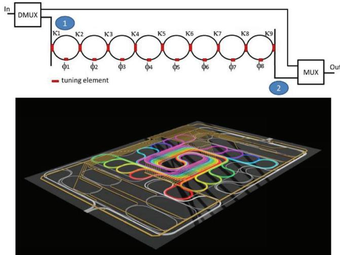
**Figure 3: functional schematics (top) and 3D model of the designed chip (bottom)**
