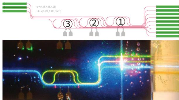
Figure 4: Mask layout and visible light propagation through ring resonators designed for a wavelength of 2.35  $\mu\text{m}$
