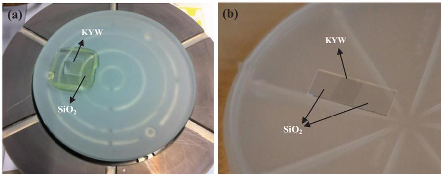
Fig. 1 (a) Mounted KYW/glass plate on metal polishing jig with vacuum; (b) Polished KYW layer on  $\text{SiO}_2$  substrate. The thicknesses of adhesive and undoped KYW layers are  $\sim 5 \mu\text{m}$  and  $\sim 2 \mu\text{m}$  respectively. The  $\text{SiO}_2$  substrate was diced from two sides to create direct accessibility to KYW layer.
