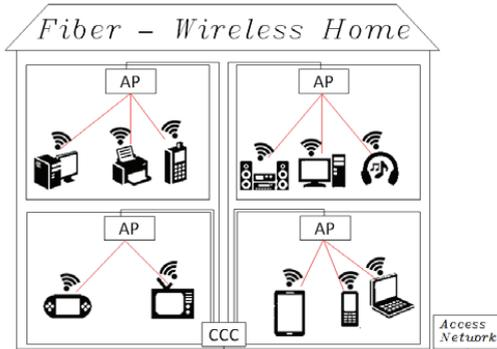
Fig. 1 Architecture of optical fiber – wireless indoor network.
