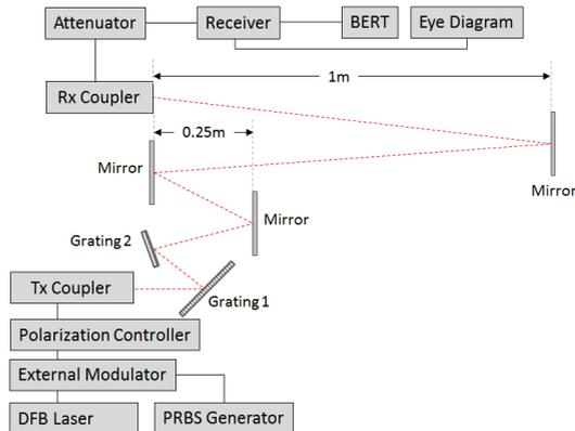
Fig. 2 Testbed setup for 2D beam-steered free-space transmission link of 2.5 m.
