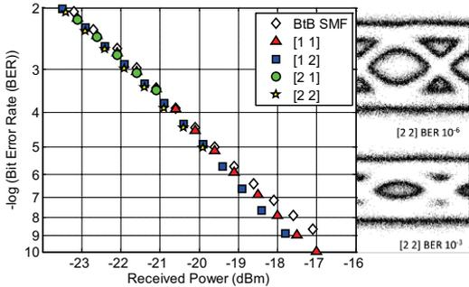
Fig. 4. Performance of 10 Gbit/s diffracted transmission links versus SMF BtB transmission. On the right is the captured eye-diagram for transmission at [2 2].
