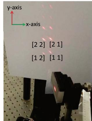
Fig. 3 2D tabulation for orthogonally cascaded echelle gratings.
