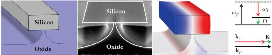
(1) A drawing, SEM-image and mechanical mode profile of the silicon wire on an oxide pillar. The color of the mechanical mode indicates the horizontal displacement (red: +, blue: -). The energy diagram and phase-matching condition of forward SBS are depicted on the right.
