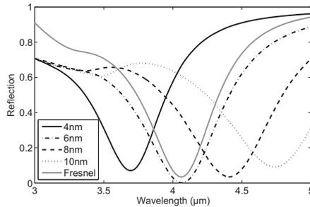
**Figure 3:** Plot of the reflection of GPs with a change of doping from  $E_{F,in} = 1\text{eV}$  to  $E_{F,cav} = 0.25\text{eV}$  at the end of a semi-infinite graphene sheet with length  $d$  indicated in the legend. Critical coupling is reached when the size of the smaller doping zone is 6nm. The grey curve stands for the Fresnel computed reflection.
