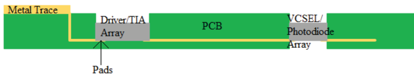
Figure 4 Assembly of flipped chips in PCB
