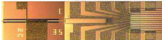
Fig. 2: Optical integrated chip of full-band tunable laser (DFB laser array, coupler and SOA).
