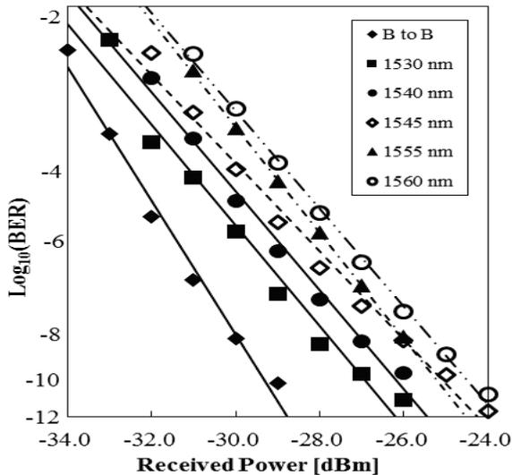
Fig. 3: Result of bit error rate test
