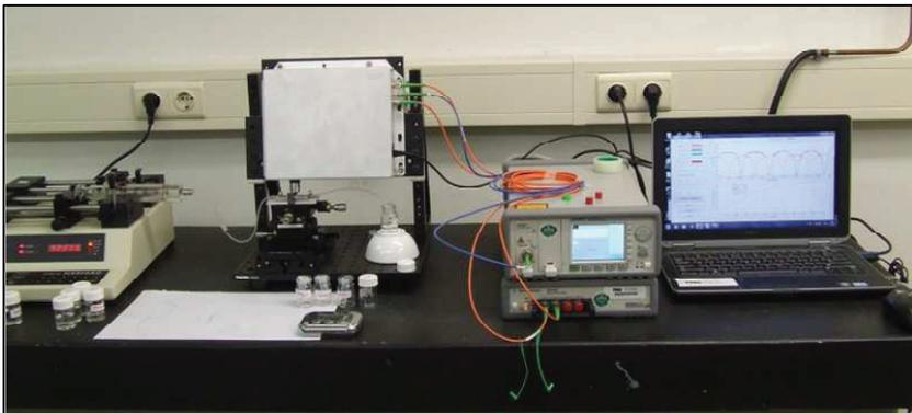
*Figure 3: the system in action in a bio-chemical test. From left to right: syringe pump, chip system, tunable laser and detector (Agilent), and laptop with dedicated software.*
