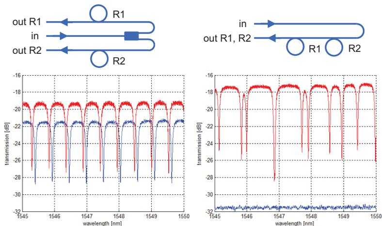
*Figure 4: typical signals for parallel rings (left) and rings in series (right). In the right figure, the blue curve corresponds to a device of which the input is not excited, and shows the system reflection.*
