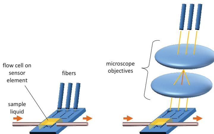
Figure 1: fiber-chip pigtailed (left) and a free-space coupling (right)
