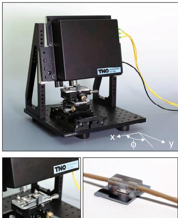
*Figure 2: photograph of desktop tool (top), a zoom-in on the sensor chip with flow cell with the stage sled forward to the chip replacement position (lower left), and a chip with flow cell (lower right).*
