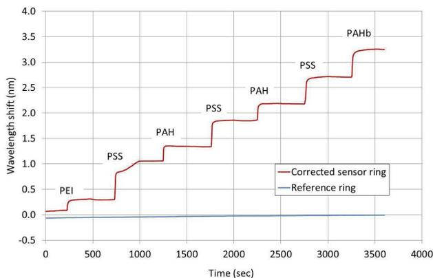
*Figure 5: binding curves of poly-electrolytes obtained using this system. system. PEI, PSS, PAH, and PAHb stand for polyethylenimine, poly(styrene sulfonate), poly(allylamine hydrochloride), and biotinylated poly(allylamine hydrochloride), respectively.*
