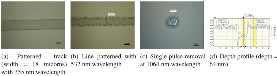
Figure 1: *Selective patterning of Plexcore thin films with 355nm, 532 nm and 1064 nm picosecond pulses.*
