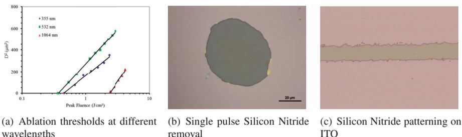
Figure 2: Ablation threshold determination for Plexcore thin films; patterning of Silicon Nitride thin films.
