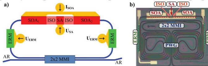
**Fig. 1.** a) Schematic diagram of the photonic integrated circuit based ring mode-locked laser: semiconductor optical amplifier (SOA), saturable absorber (SA), electrical isolation (ISO), electro refractive modulator (ERM) and multi-mode interference coupler (2x2 MMI) sections and passive waveguides in blue b) A microscope image of the fabricated device.
