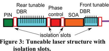
Figure 3: Tuneable laser structure with isolation slots.
