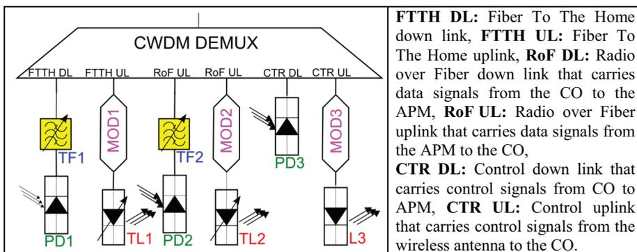
**Figure 1:** Scheme of the proposed chip design.
