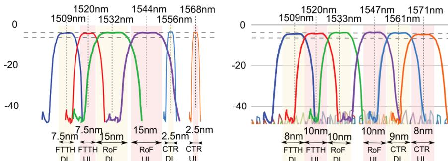
Figure 2: Comparison of the target and designed spectral response of the multi/demultiplexer
