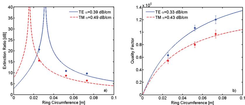
**Figure 4:** Measured ring resonators with different circumferences: (a) Extinction Ratio, (b) Quality Factor.
