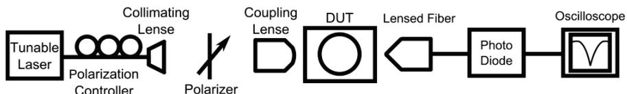
**Figure 3:** Schematic of the experimental setup to measure the ring transmission.
