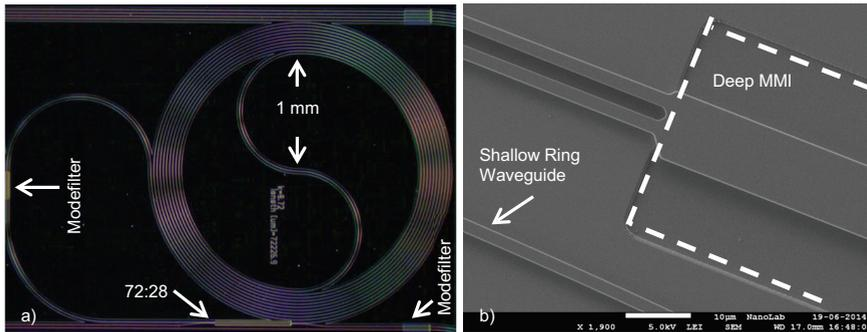
**Figure 2:** (a) Microscope picture of a MMI coupled spiral ring resonator with 73 mm circumference. (b) SEM image of 72:28 MMI used for coupling.
