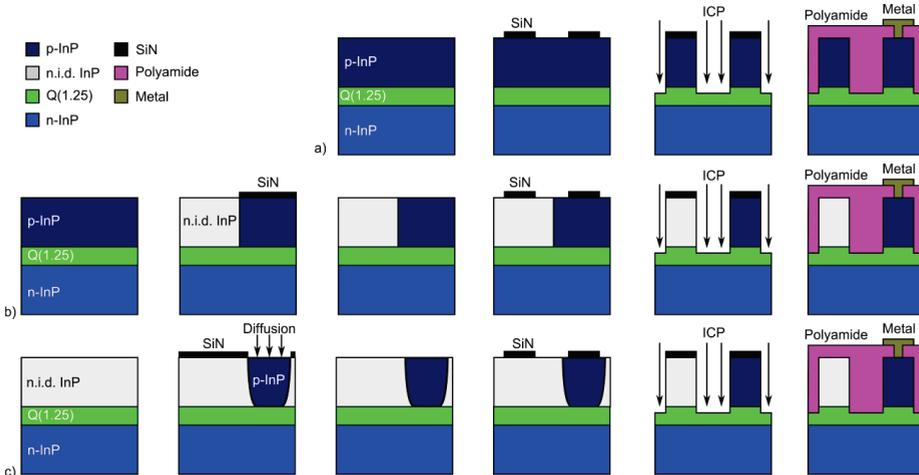
**Figure 1:** Schematic of waveguide fabrication using: (a) PIN substrate, (b) PIN substrate with regrown n.i.d. top cladding, (c) n.i.d. substrate with doped cladding formed by local Zn-Diffusion.
