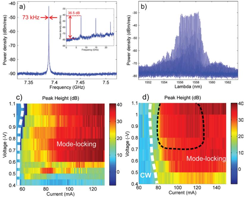
Figure 2. a) RF spectrum recorded at  $I_{SOA} = 96$  mA and  $U_{SA} = -0.6$  V for the case when absorber is placed to the low reflectivity output mirror. Inset: Broadband RF spectrum showing second and third harmonics. b) The optical spectrum at the same operating conditions as in (a). A map of the RF peak height as a function of bias conditions measured for the case when SA is placed at the output coupler (a) and when SA is at the end mirror (b).
