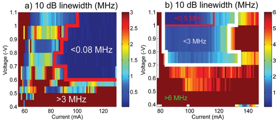
Figure 3. A map of the RF linewidth measured at 10 dB level for the case when SA is placed at the output coupler (a) and when SA is at the end mirror (b).
