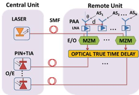
Fig.1. Optical beamforming system architecture
