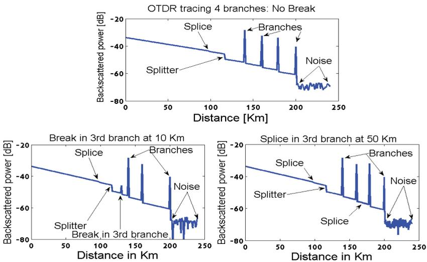
**Figure 1:** OTDR tracing for 4 branches (a) No break. (b) With break in 3rd branch. (c) With splice in 3rd branch.
