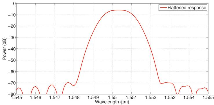
Fig. 4: Central output waveguide response
