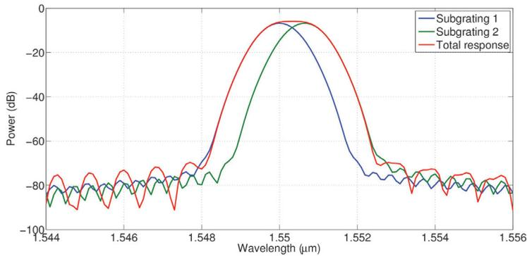
Fig. 2: Simulated AWG as two subgratings and using both AW groups at the same time
