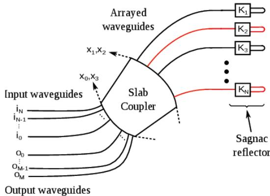
Fig. 1: Reflective AWG schematic. There exists an incremental length between arrayed waveguides in the same group. Different colors stand for different AW groups. Abbreviations:  $K$  stands for coupling constant and  $x$  stands for spatial AWG planes.
