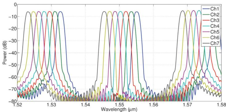
Fig. 3: Transfer function from central input waveguide to the output waveguides
