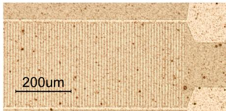
**Figure 5:** Fabricated IDTs on a waveguide chip
