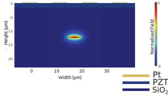
**Figure 1:** Cross section of the waveguide and IDT structure. The intensity distribution cross section of the  $TM_{00}$  for 840 nm wavelength is superimposed. All shown features are to scale.
