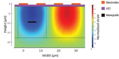
**Figure 2:** Cross section of calculated strain distribution of the fundamental surface acoustic wave, displayed over one acoustic wavelength. The size of the waveguide and IDTs are exaggerated for clarity.
