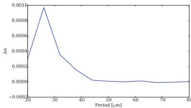
**Figure 3:**  $\Delta n_{eff}$  of the  $TM_{00}$  mode in the waveguide for a wavelength of 840 nm as a function of the acoustic wavelength, at a driving voltage of 6 V.
