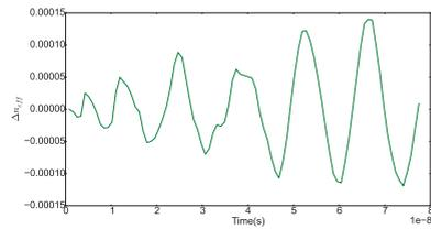
**Figure 4:** Dynamical evolution of the effective refractive index for an IDT period 44  $\mu\text{m}$  excited with 73.4 MHz.
