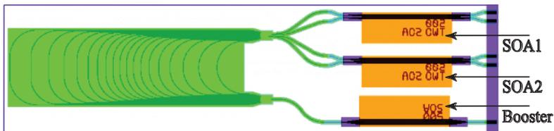
Fig. 3. Mask layout of 0.65 mm × 2.75 mm 4-channel AWG-based laser. This device has two SOAs: SOA1 and SOA2, each of which has two parallel waveguides connected to different ports (channels) of the AWG. Four different wavelengths can be generated using just two SOAs. Note that the booster amplifier is inside the FP-cavity. The cavity is formed between the cleaved facet.
