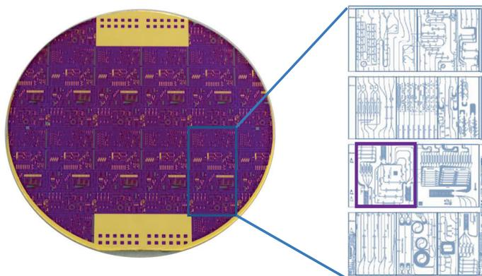
Figure 1. Multi project InP 3" wafer filled with application specific photonic ICs, processed at Oclaro. Versatile photonic devices can be fabricated in single technological processes.
