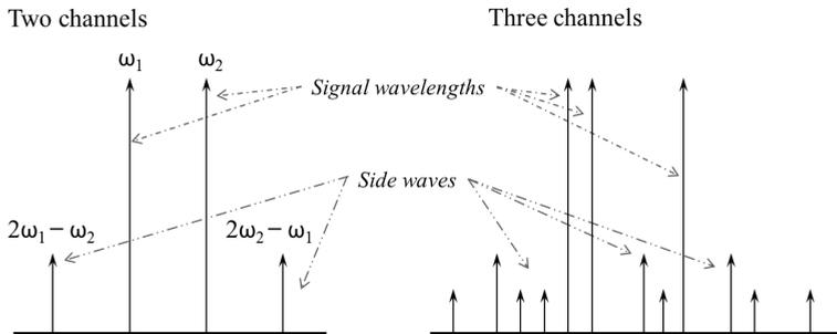
Fig. 2. Four-wave mixing effect in two and three channels systems. The interaction between signal wavelengths in a nonlinear medium results in creation of side waves.
