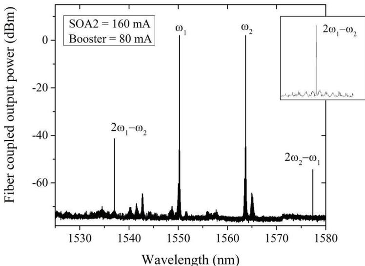
Fig. 4. FWM effect observed in the booster amplifier of the 4-channel AWG-based laser. The peaks corresponding to the  $\omega_1$  and  $\omega_2$  were generated by the SOA2, and correspond to two different AWG channels, spaced by two free spectral ranges of AWG. The two side peaks,  $2\omega_1 - \omega_2$  and  $2\omega_2 - \omega_1$ , are the effect of FWM, with the output power more than 40 dB lower than the signal wavelengths.
