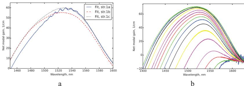
Figure 2: Calculated net modal gain. (a) Comparison of gain calculated with three structures. (b) Gain for different pump currents measured on the structure of fig. 1c.
