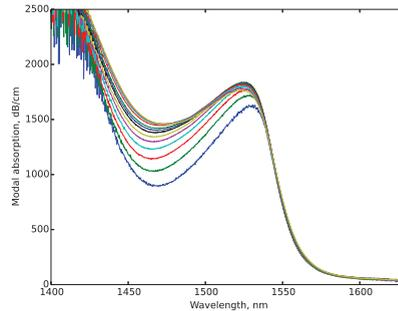
Figure 3: Calculated SOA absorption spectra. Different curves correspond to different levels of  $P_{in}$
