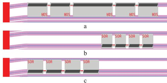
Figure 1: Mask layout of MS-SOAs. Lengths of sections: (a)  $L_{\text{SOA}} = 200, 200, 400, 200, 200 \mu\text{m}$ . (b)  $L_{\text{SOA}} = 100 \mu\text{m}$ . (c)  $L_{\text{SOA}} = 150 \mu\text{m}$ .
