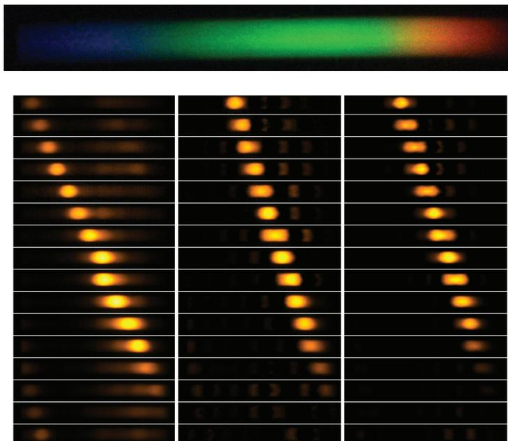
Figure 3 Rainbow pattern recorded with standard RGB camera (top). Hyperspectral datacube recorded on mosaic sensor (bottom): original data (left), data after linear transformation (middle) and data after non-linear transformation (right)
