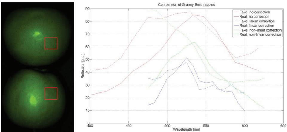
Figure 4 Spectral comparison measurement between fake (left: top) and real apple (left:bottom) represented by relative spectral response in part of the image (right).
