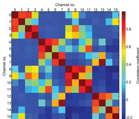
Figure 2 Cross-talk scheme on mosaic sensor represented via correlation coefficients between channels
