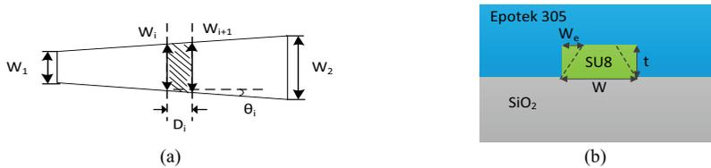
Fig 1: (a) Top view of linear taper; (b) Cross section profile. The green rectangle was the intended shape while the dotted lines show the actual shape of the experimental waveguides.
