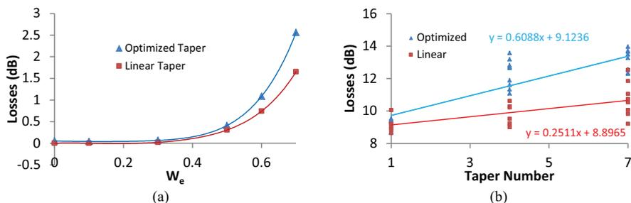
Fig 4: (a) Simulated taper losses as a function of etched width  $W_e$ , and (b) measured total losses as a function of number of tapers. The slope of the linear fits represents the total losses per taper. Both simulation and measurement were realized at the wavelength of 1.3  $\mu\text{m}$  wavelength.
