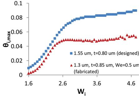
Fig 2: The maximum tapering angle calculated at the wavelength of 1.3  $\mu\text{m}$  (red) and 1.55  $\mu\text{m}$  (blue).
