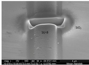
Fig 3: SEM image of the cross section profile.
