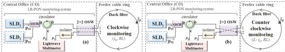
Fig. 1. Schematic diagram of the proposed TRA based monitoring solution. (a) Clockwise direction. (b) Counter clockwise direction
