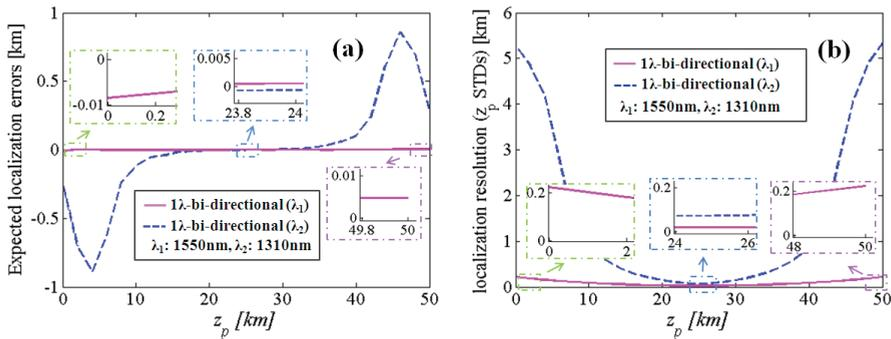
Fig. 3. (a) Calculated expected localization errors and (b) Corresponding STDs when a fiber bending/seepage is introduced along the feeder ring.
