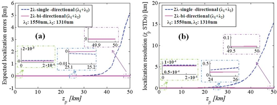
Fig. 2. (a) Calculated expected localization errors and (b) Corresponding STDs when a fiber break is introduced along the feeder ring.
