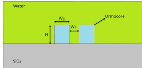
Figure 1: Cross-section of the slot waveguide
