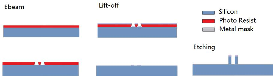
Figure 4: fabrication of master mold
