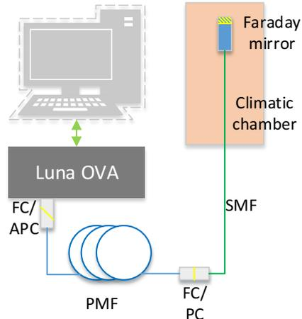
Figure 3. Scheme of the experimental setup to measure  $PMD_{FRM}$ .
