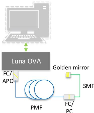
Figure 2. Scheme of the experimental setup to measure  $PMD_{PMF}$ .
