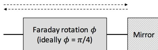
Figure 1. Internal schematic of the Faraday mirror.
