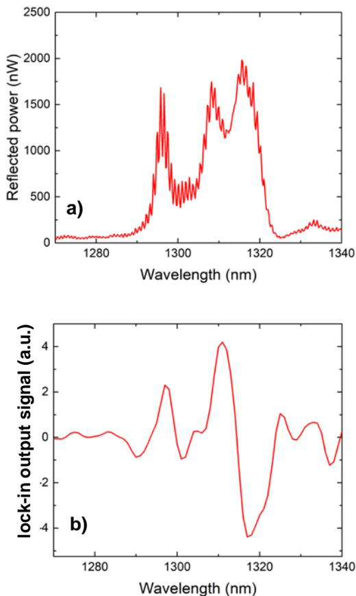
*Figure 4:* a) Optical reflectivity spectrum measured through the fiber. b) Lock-in output signal referenced by the 4.3 kHz frequency of the transducer drive voltage.
