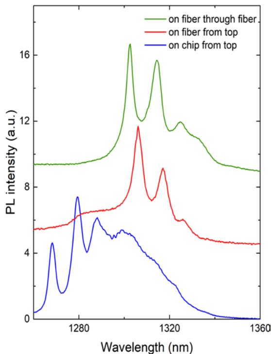
Figure 3: PL-spectra of DM structure. Blue (bottom): as on chip before picking. Red (middle) and green (top): after mounting on the fiber tip, from the free space side with an objective (red) and from the fiber side (green)
