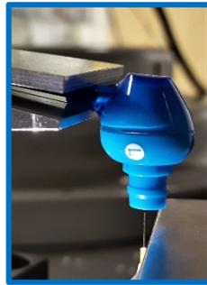
*Figure 5:* Experimental setup used to measure the mechanical displacement introduced by applying a sound wave using an audio speaker. *Inset:* Picture of the headphone speaker placed above the fiber tip.
