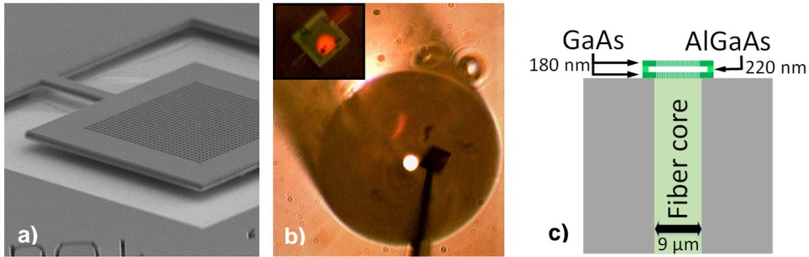
Figure 2: a) SEM image of the fully released DM structure on chip. b) Fiber tip & nanomanipulator during pick&place procedure. Inset: Top view of device placed on fiber core with red laser applied via the fiber (note some misalignment). d) Schematic side view of DM on fiber core (not to scale).
