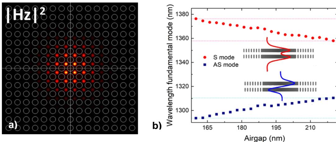
*Figure 1: a) Simulated circular shaped  $|H_z|^2$  field pattern of the fundamental mode. b) Calculated tuning curve of the fundamental symmetric (S) and anti-symmetric (AS) mode of the double membrane structure.*
