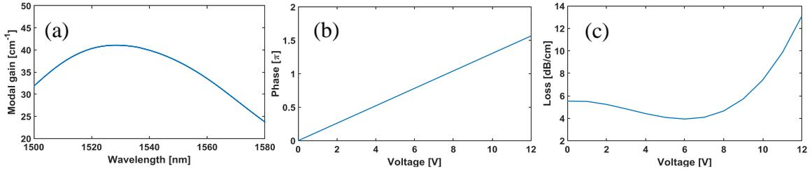
Figure 1. (a) SOA modal gain for current density 2.5 kA/cm<sup>2</sup>, (b) Phase shift for 1 mm long ERM as a function of voltage, (c) Loss per unit length as a function of voltage for ERMs from experimental results.
