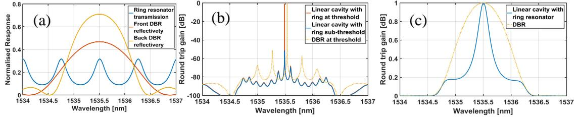
Figure 3. (a) Response of ring resonator and DBR gratings, (b) Spectra of linear laser with ring resonator below threshold (blue) and at threshold (orange) and DBR laser at threshold (yellow dashed line), (c) total filter response of linear cavity with ring resonator and DBR laser (blue and dashed yellow respectively)
