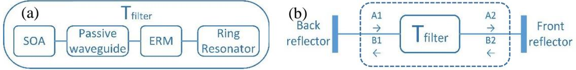
Figure 2. (a) Example of an intra-cavity filter and definition of the total T-matrix, (b) forming the cavity using two reflectors.
