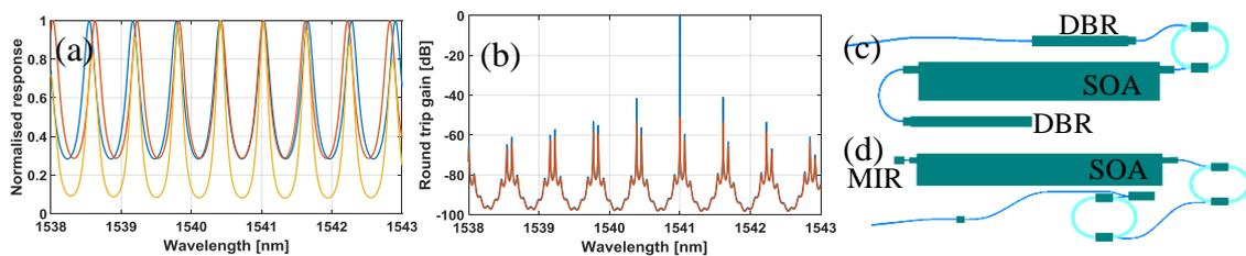
Figure 4. (a) Ring resonators transmission spectra (blue and orange) and total filter response (yellow), (b) Spectra of Vernier laser below threshold (orange) and at threshold (blue), (c) Linear cavity laser design with DBRs and ring resonator, (d) Linear cavity laser based on Vernier effect
