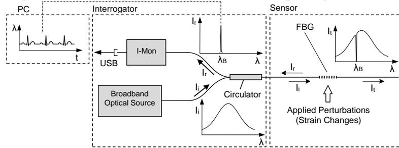
Fig. 2. Interrogation system of the FBG-based sensor network.
