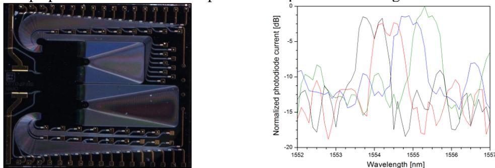
Fig. 3. The microscope picture of the AWG-based integrated interrogators (left) and the measured transmission characteristic of the 50 GHz AWG wavelength demultiplexer (right).
