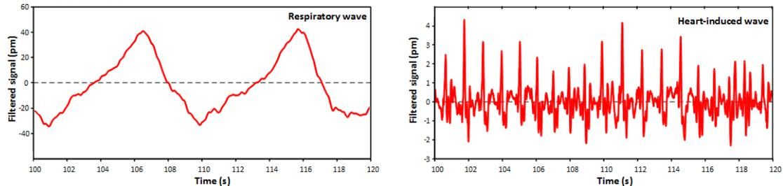
Fig. 4. Measurement results obtained using the test setup - respiratory and heart-induced waves plotted as a function of the deviation of the Bragg wavelength in the time domain.
