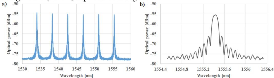
Fig. 1. Measured reflected spectra of six FBGs written in hydrogen-loaded fiber (left) and the detailed spectrum of a single FBG (right).
