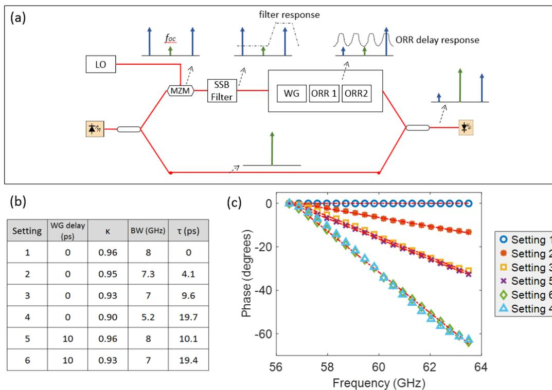
Figure 3. (a) Schematic diagram of the system for simulation; (b) Different beamformer settings and the corresponding delay; (c) Phase response for different beamformer settings.
