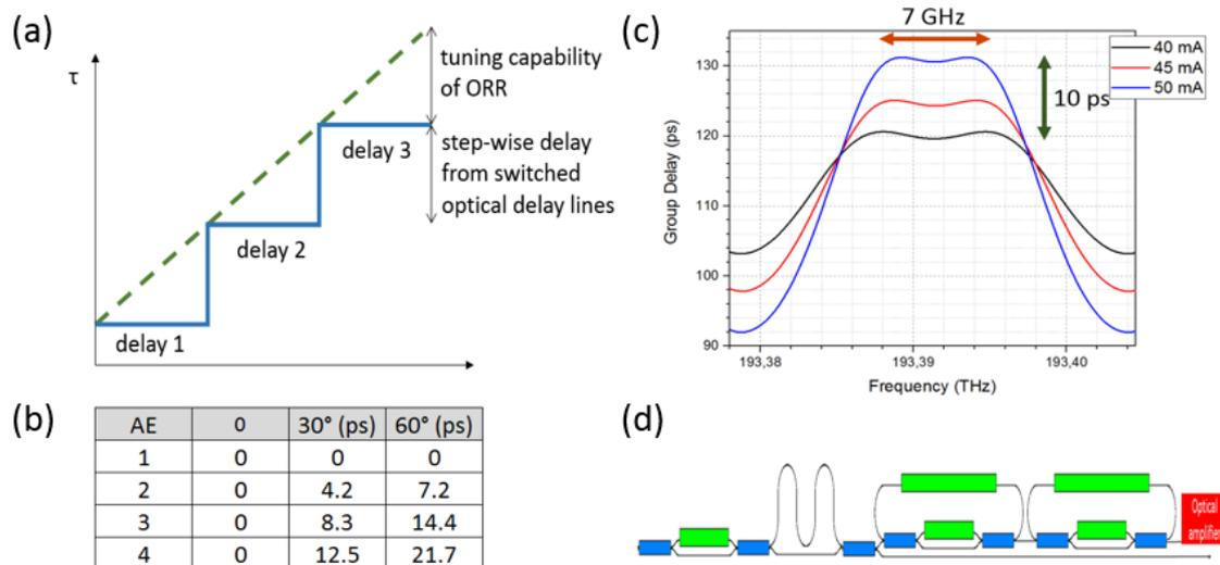
Figure 2. (a) Principle of operation; (b) Delay values for a 4x1 PAA; (c) Group delay response for two cascaded ORRs; (d) Schematic of the ORR-assisted true time delay employing switched delay lines.
