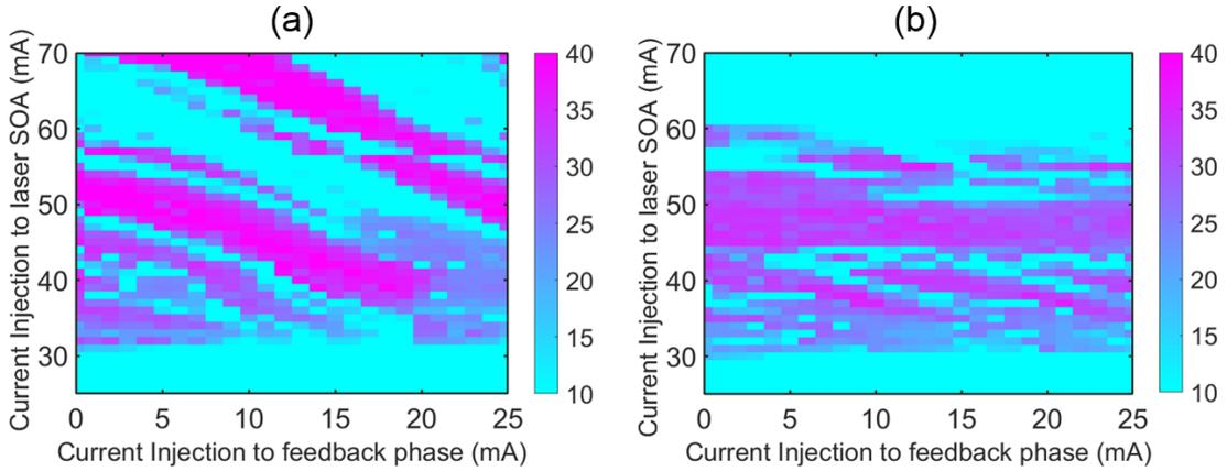
**Fig. 4:** Measured stability map for feedback phase of the (a) short and (b) long feedback path, the color bar shows the SMSR in dB.
