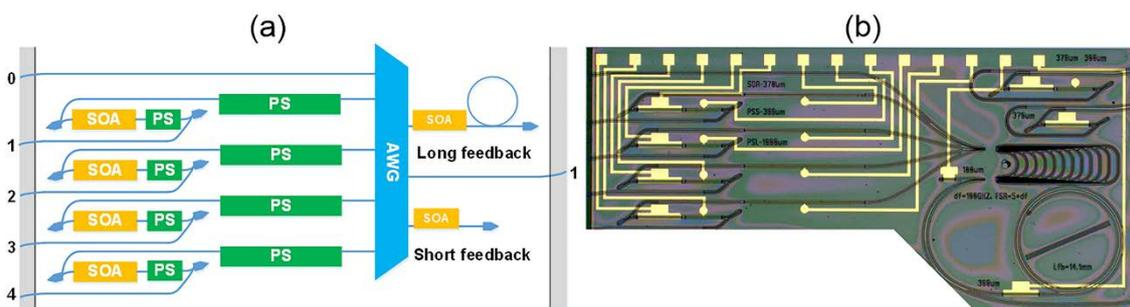
**Fig. 1:** (a) Schematic diagram and (b) microscope photograph of a filtered feedback multi-wavelength laser.
