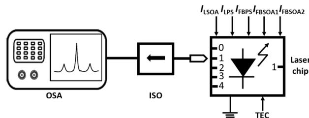
**Fig. 2:** The measurement setup.  $I_{LSOA}$ ,  $I_{LPS}$ ,  $I_{FBPS}$ ,  $I_{FB SOA1}$ ,  $I_{FB SOA2}$  represent forward/reverse bias that are driven to the electrical contacts of SOAs and phase shifters; the numbers represent the I/O ports of the device; TEC is the temperature controller; ISO is an optical isolator; OSA is an optical spectrum analyzer.
