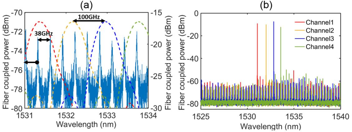
**Fig. 3:** (a) A zoom of the spectrum of the FP laser at subthreshold and the estimated AWG filtering function for each laser with the long feedback on. (b) Superimposed lasing spectra of the four channels while operating each channel separately.
